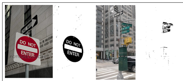
Figure 4.1: Dynamic thresholding in the HSL space for red and green
